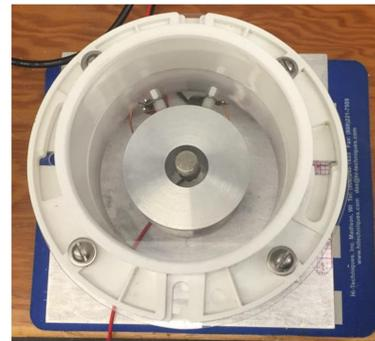
Fig. (A,B,C) 4.5 inch diam SPO (two PVC flanges, 1/8 inch clamped acrylic plate, rare earth magnet (1cm diam) and accelerometer on underside. Fig. (D) 8.0 inch diam alum. SPO.
