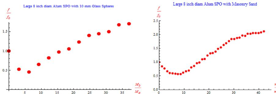
Figure 3. Comparing resonant frequency vs. mass loading in an 8 inch diam SPO with A clamped plate mass  $M_p = 108$  grams. (A) 10 mm glass spheres, (B) sifted masonry sand
