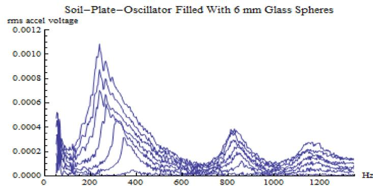
Figure 1. A set of tuning curve responses of a Soil Plate Oscillator (SPO) filled with 6 mm glass spheres. The clamped acrylic 1/8 inch plate is 4.5 inch in diam.
