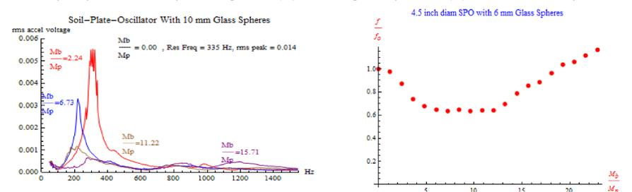
Figure 4. Comparing resonant frequency vs. mass loading effects in a 4.5 inch diam SPO
